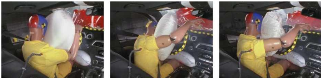
Fig. A.2 Example of Partial Frontal Airbag Action
