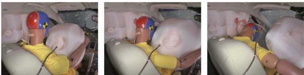
Fig. A.6 Example of Little Frontal Airbag Action
