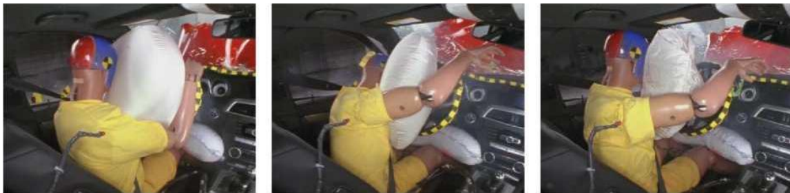
Fig. B.2 Example of Partial Frontal Airbag Action
