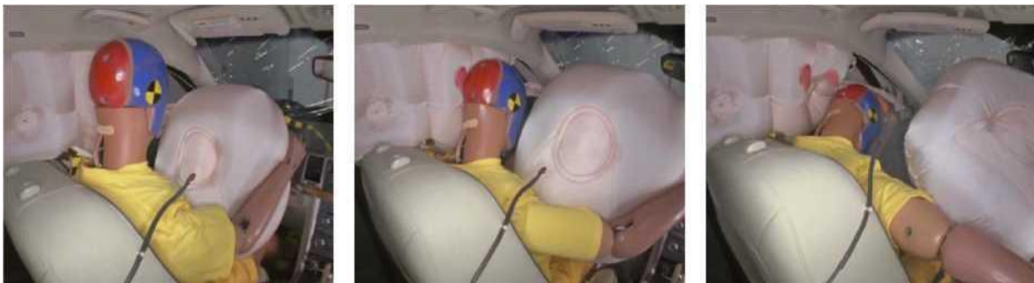
Fig. B.6 Example of Little Frontal Airbag Action
