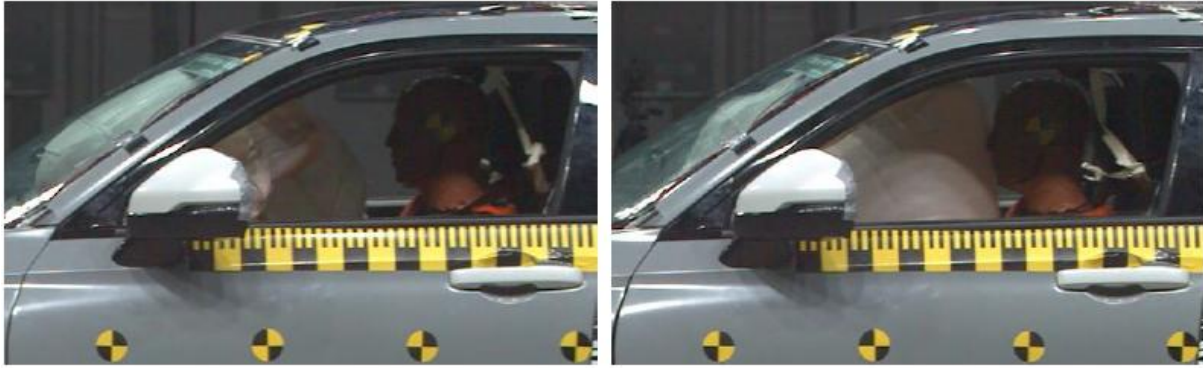
Fig. C.2 Example of Dangerous Deployment of Frontal Airbag
