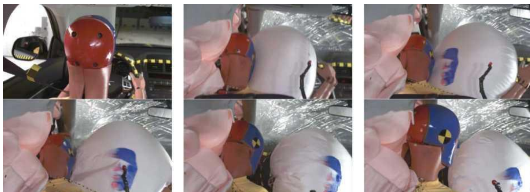
Fig. A.3 Example of Partial Frontal Airbag Action
