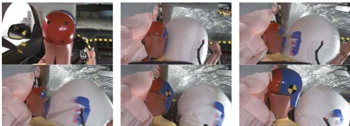
Fig. B.3 Example of Partial Frontal Airbag Action
